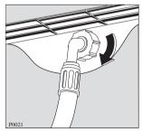
If necessary turn the hose adequately by unscrewing the nut at the rear of the appliance. Now tighten the nut anew to avoid leaks. (Open the tap and assure that it does not leak and close it again.)
